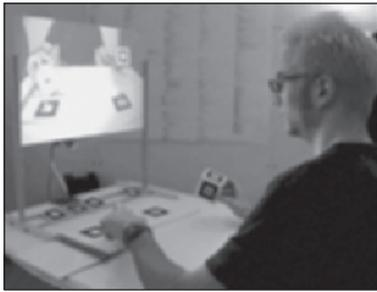
**Figure 3.** System set-up with a typical situation of use: charging the Gripper with an element from the booklet (left). The platform (right) holds an unsaturated atom, with which a binding with the charged atom may be triggered (Fjeld & Voegtli, 2002). Image by courtesy of Morten Fjeld and Benedikt M. Voegtli.
